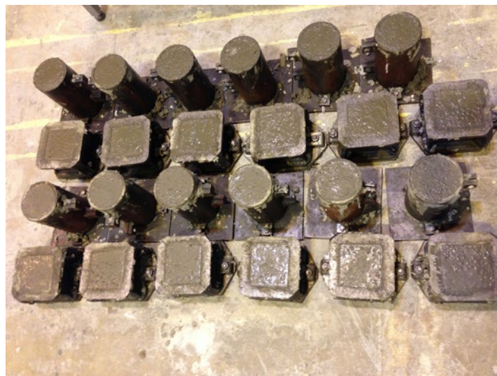
Figure 2.3 Specimen casting (12 cubes and 12 cylinders for each mix)
