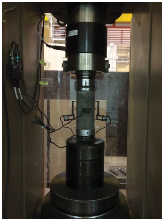
Figure 2.5 Experimental setup for modulus of elasticity test (static)
