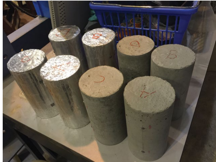
Figure 2.6 Concrete specimens for autogenous and total shrinkage test
