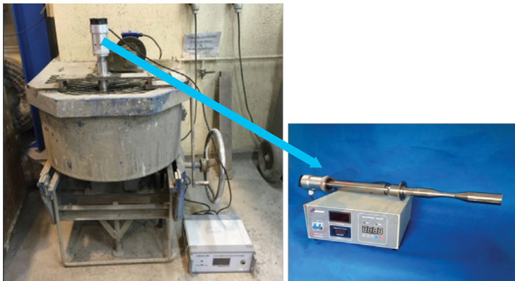
Figure 3.10 Experimental setup for ultrasonic mixing technique
