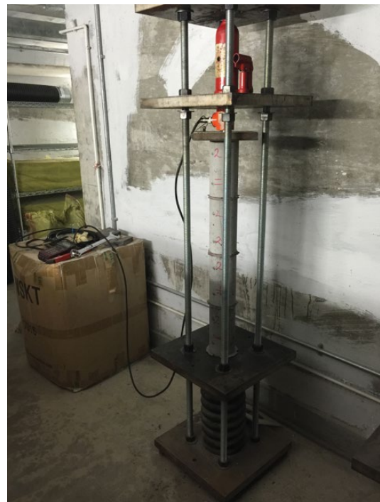
Figure 2.7 Experimental setup for creep test
