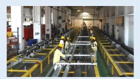
Horizontal Pipe Modules under Fabrication at Factory
