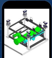
Phase 3 Install first layer pipework c/w accessories
