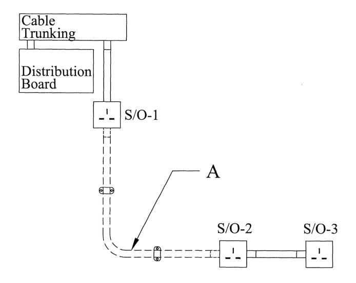
Drawing No.1 – Wiring diagram of a Radial Circuit of 13A Socket Outlets
