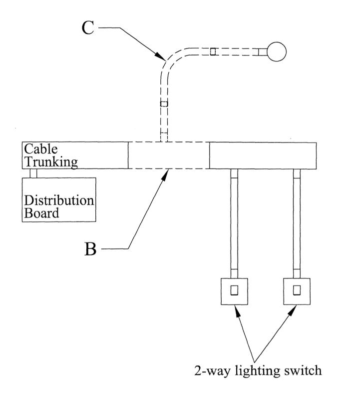
Drawing No.2 – Wiring diagram of a lighting final circuit with 2-way switching
