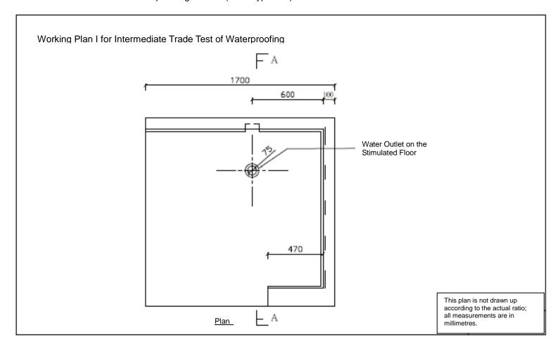
Working Plan II for Intermediate Trade Test of Waterproofing Worker (Burn-Type Felt)
