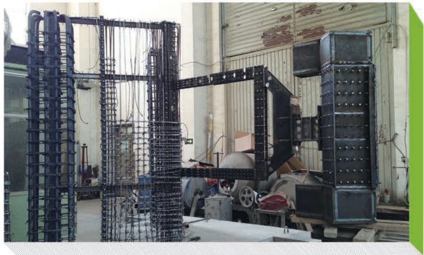
Figure 6: The experiment model of outrigger wall system
