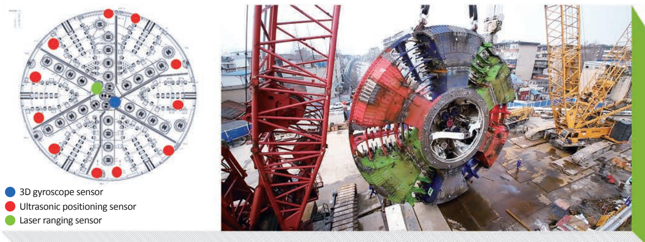
Figure 4: Layout of sensors on cutter wheel
