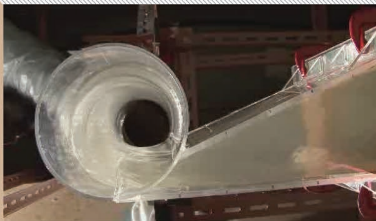
Figure 9: Air core of the tangential vortex intake.
