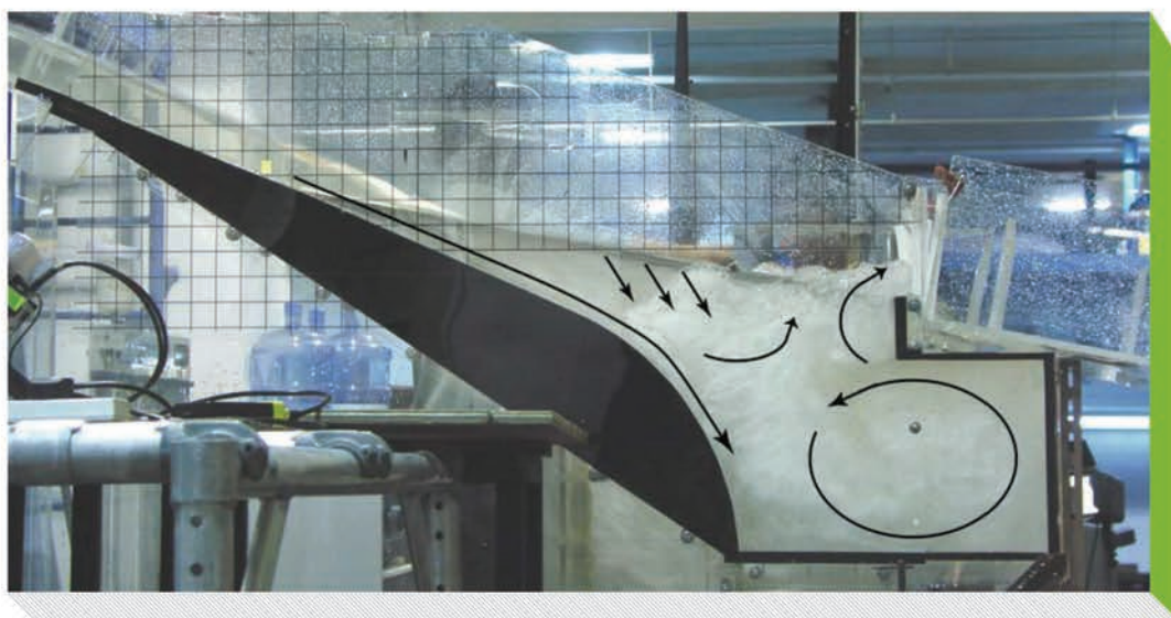
Figure 5: Bottom rack intake for supercritical flow diversion (final design); observed flow at Q = 53.9 L/s.
