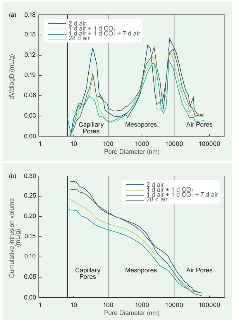
Figure 3. Pore size distribution (MIP) of cement-bonded particleboards produced by different curing methods: (a) differential distribution; (b) cumulative distribution
