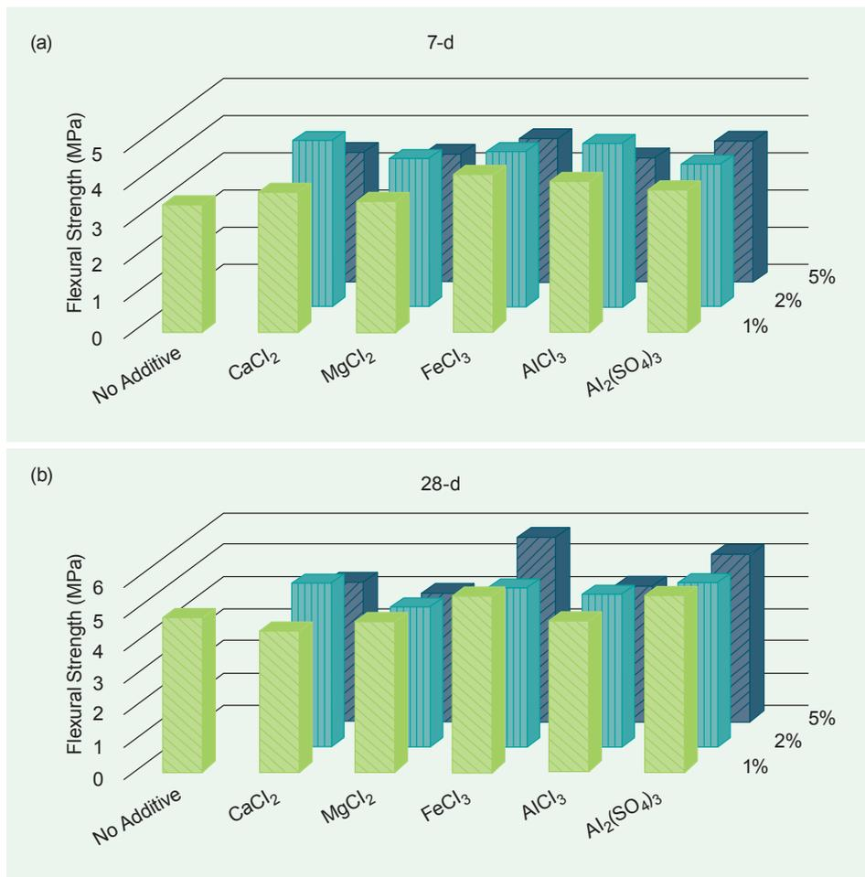
Figure 1. Flexural strength of cement-bonded particleboards with various accelerators at different dosages: (a) 7-d curing; (b) 28-d curing.
