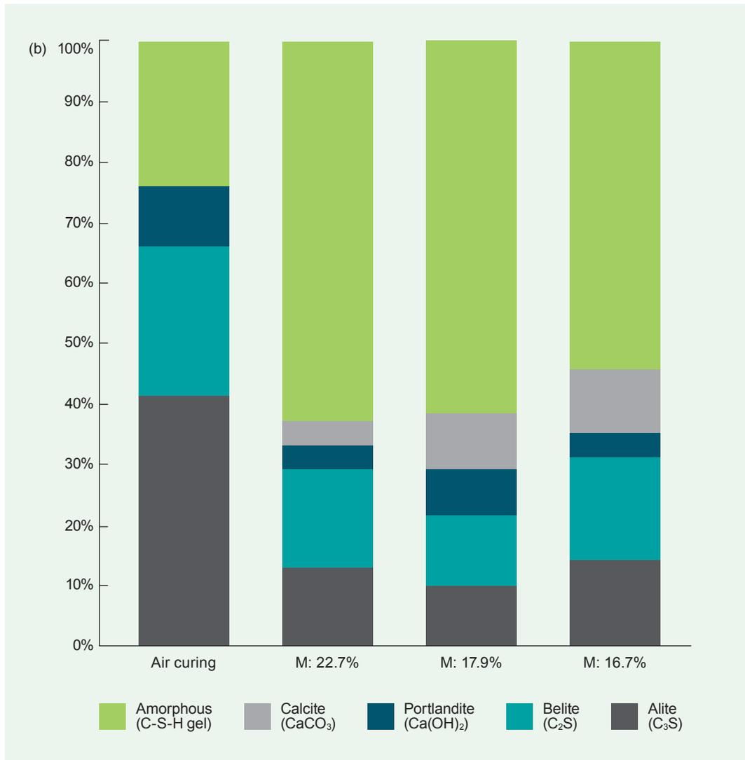
Figure 4. XRD spectra (a) and XQRD analysis (b) of cement-bonded particleboards produced by different curing approaches (M: moisture content).
