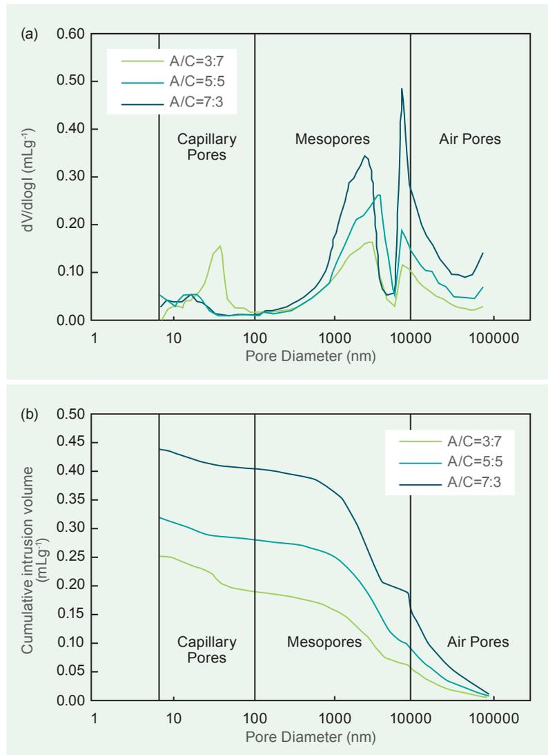
Figure 2. Pore size distribution (MIP analysis) of 28-d particleboards at varying aggregate-to-cement (A/C) ratio:(a) differential distribution; (b) cumulative distribution
