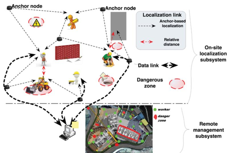
Fig 3 The overview of the RTLS to be developed
