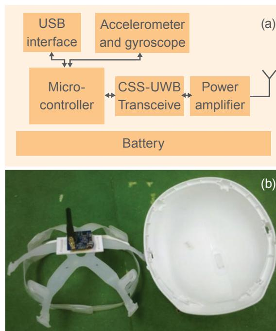
Fig 1 (a) The hardware design of the s-Helmet (b) The s-Helmet
