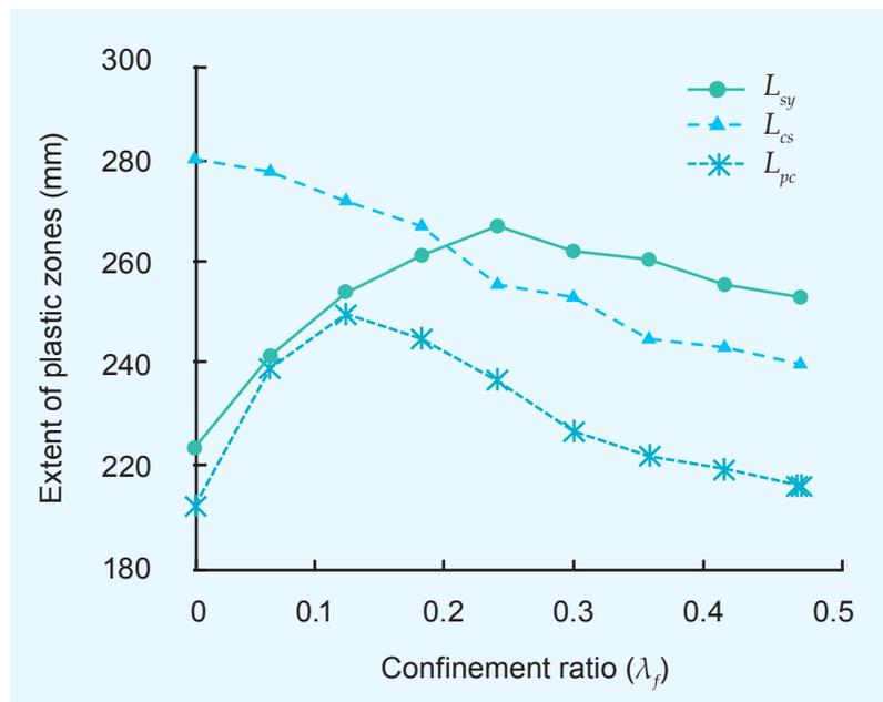
Figure 7 Effect of the confinement ratio on the plastic hinge lengths
