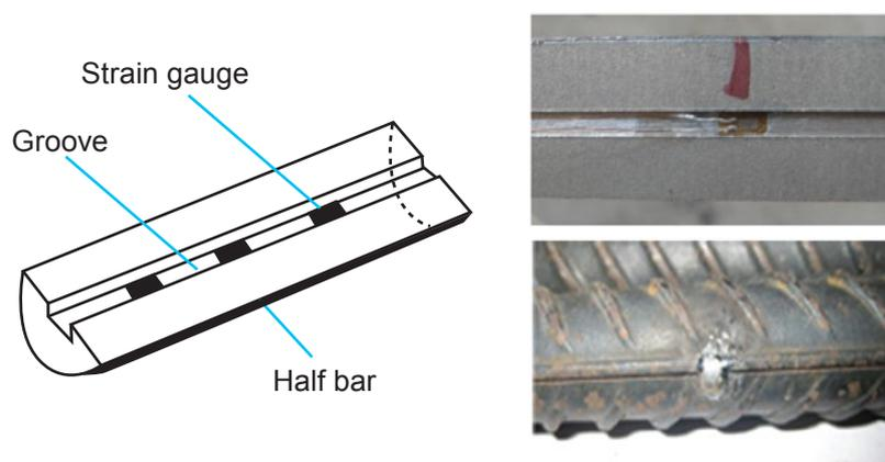
(b) Strain gauge installation in the steel reinforcing bars
