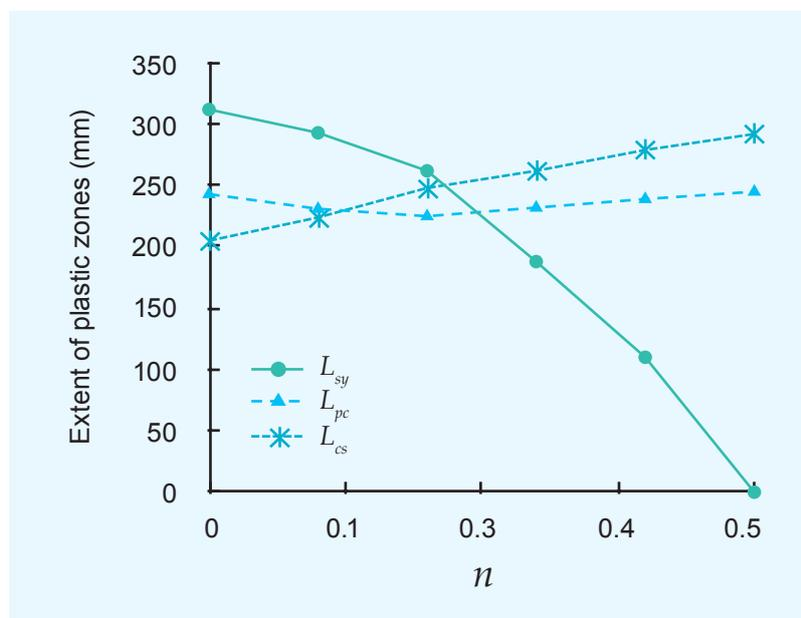
Figure 9 Effect of the axial load ratio on the plastic hinge lengths
