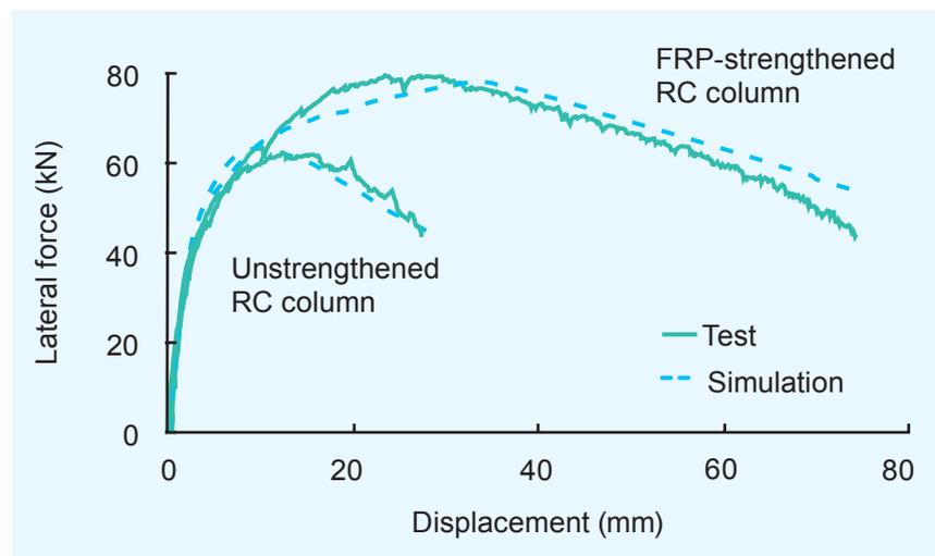
Figure 6 Calibration of the FEM model
