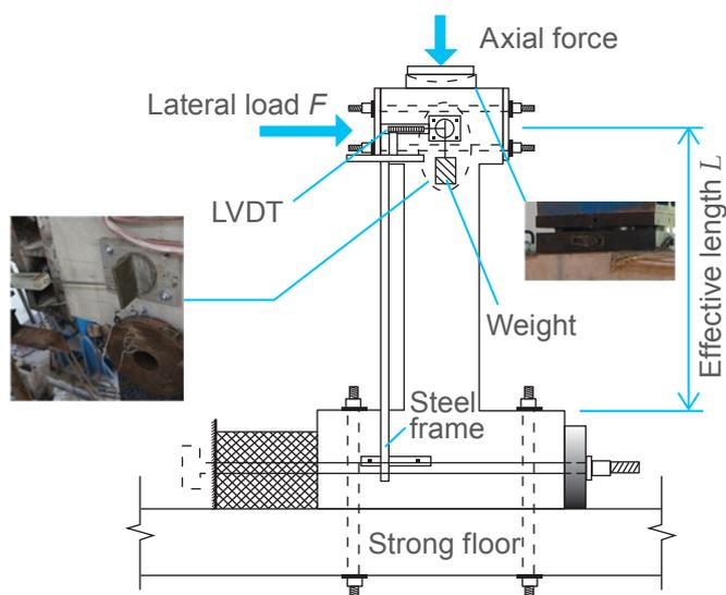
Figure 1 Typical setup of column tests
