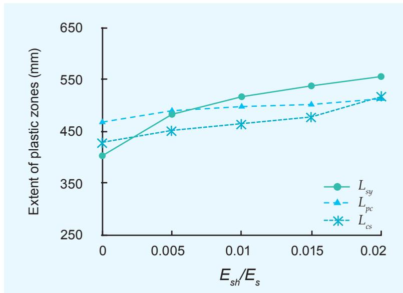
(c) effect of the hardening modulus of steel
