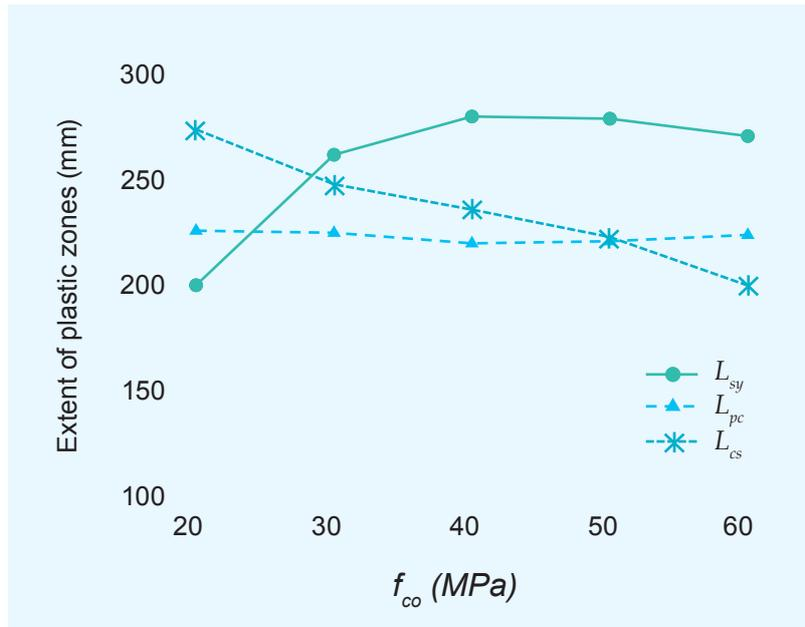
(b) effect of the compressive strength of concrete
