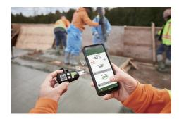
The sensors measure the temperature of concrete in real-time and can estimate the early-age and compressive strength of in-place concrete based on the maturity method.
