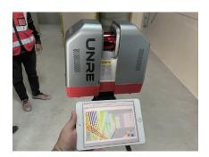
A lidar-based scanning device with built-in 3D data algorithmic processing to extract measurement information in real time.
