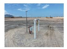
4DBloc is a GNSS based receiver designed to be deployed on construction site for long-term movement monitoring.
