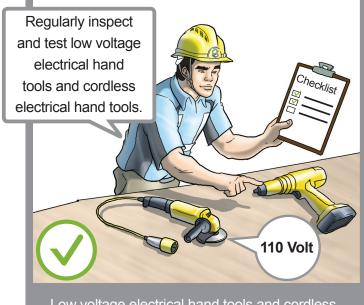
Low voltage electrical hand tools and cordless electrical hand tools should be inspected and tested regularly by a competent person.
