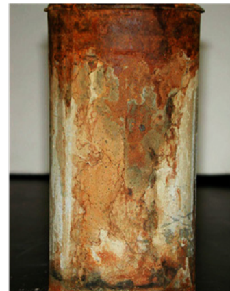
Figure 5 (a) Spalled mortar specimen after 95 hours accelerated corrosion, and (b) ECC specimen after 350 hours accelerated corrosion.
