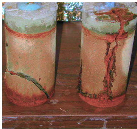
Figure 5 (a) Spalled mortar specimen after 95 hours accelerated corrosion, and (b) ECC specimen after 350 hours accelerated corrosion.
