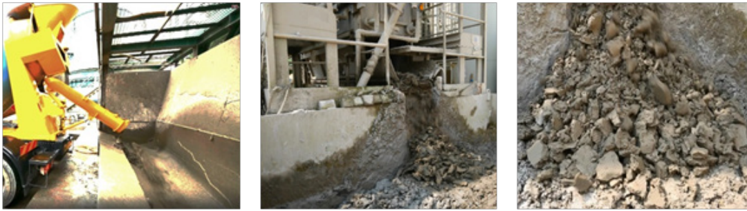
Figure 2 CSW generation at a ready-mixed concrete plant in Hong Kong
