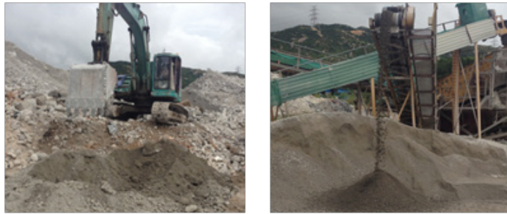
Figure 1 Production of RCAs at a C&D waste recycling plant in Hong Kong
