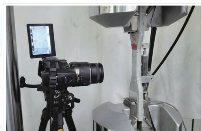
(a) Set-up of direct tension test with camera
