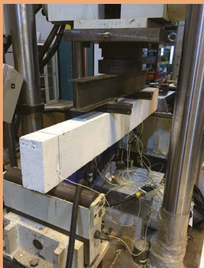
Figure 3: Experimental set-up for reinforced concrete beam bending test 圖3：鋼筋混凝土樑彎曲測試實驗裝置
