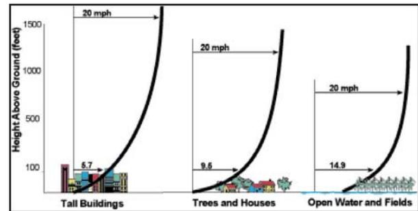
Figure 13 Typical wind speed profiles for height above ground
