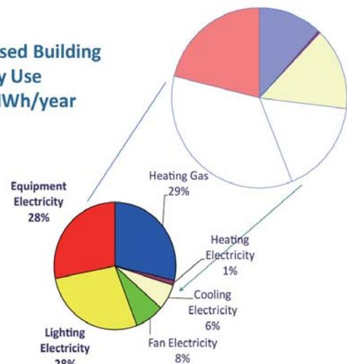
**Figure 6** 40% energy reduction in US–China Demonstration Energy-Efficient Office Building from architect’s preliminary design
