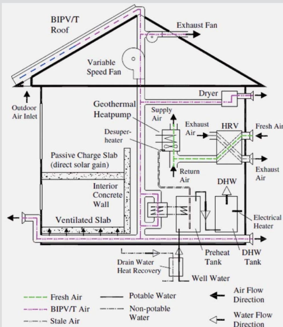
Figure 7 Applying thermal energy of the heated air from BIPV/T (adapted from Chen *et al.*, 2010)
