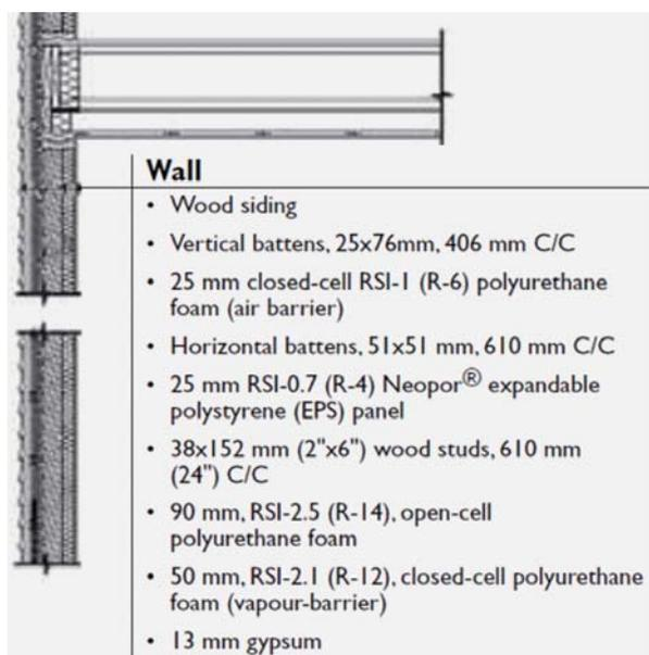
**Figure 3** Construction details of the wall assembly (CMHC, 2011a)
