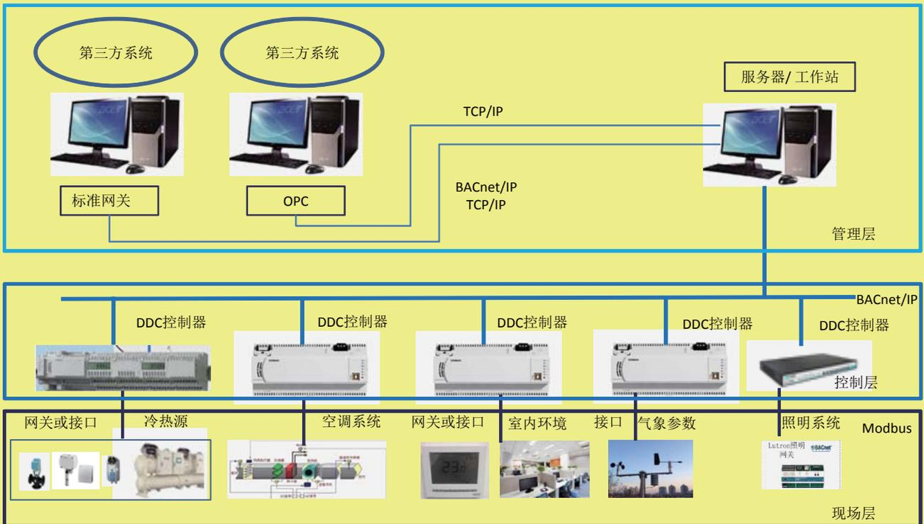
Figure 21 Construction of BAS system interface
