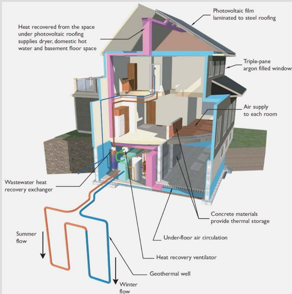
**Figure 2** Innovative technologies deployed at the EcoTerra™ house (CMHC, 2007a)
