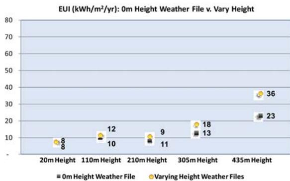
Figure 17 Heating Coil (DOAS) consumption (kWh/m²/yr)
