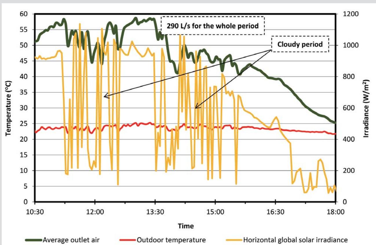
**Figure 9** Relationship between outlet temperature, outdoor temperature, and solar radiation in March (top) and in June (bottom) (adapted from Chen *et al.*, 2010)
