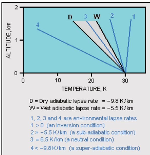
Figure 12 Different lapse rates depending on atmospheric conditions
