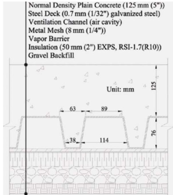
**Figure 5** Cross-section of the VCS (CMHC, 2011b)
