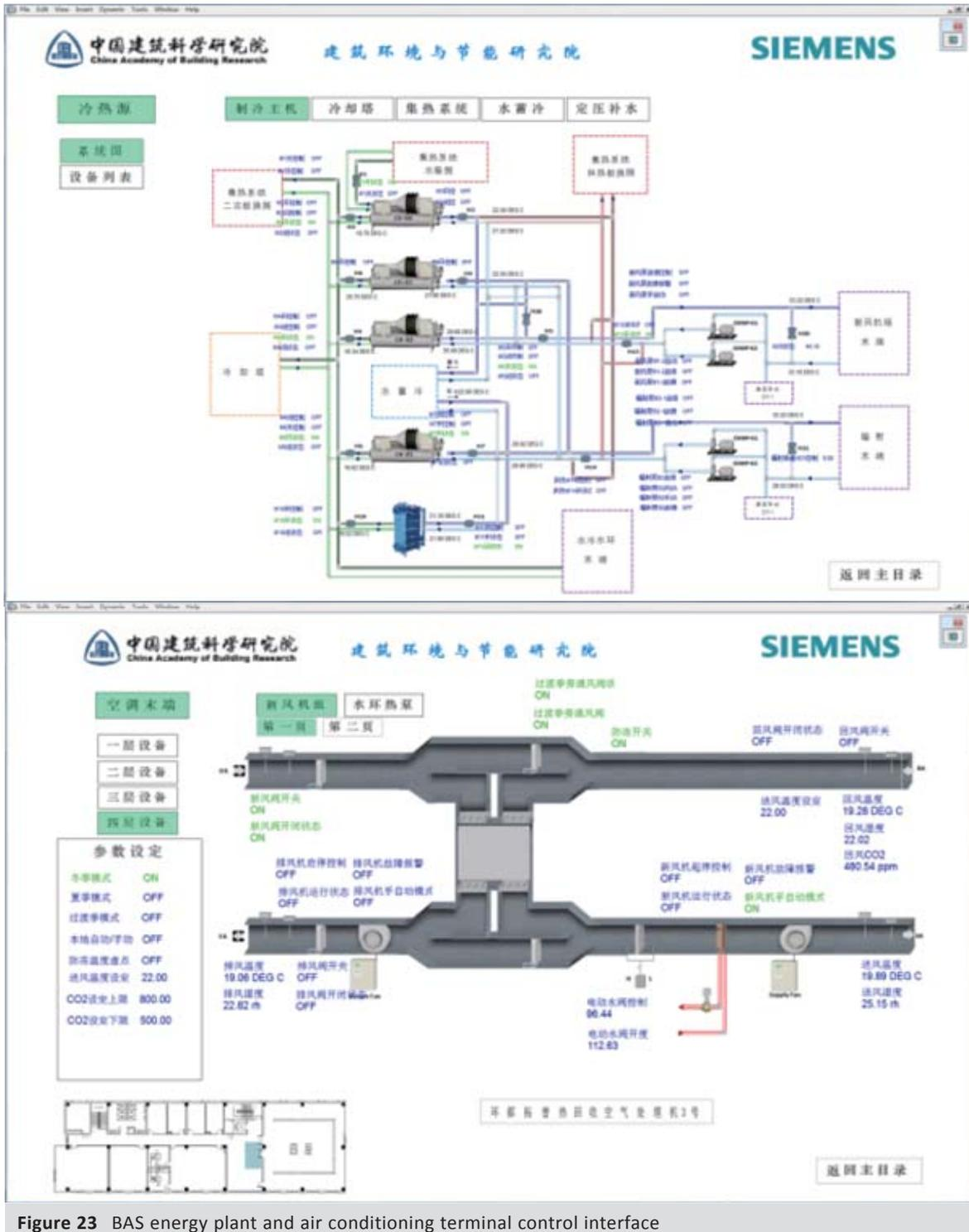
Figure 23 BAS energy plant and air conditioning terminal control interface
