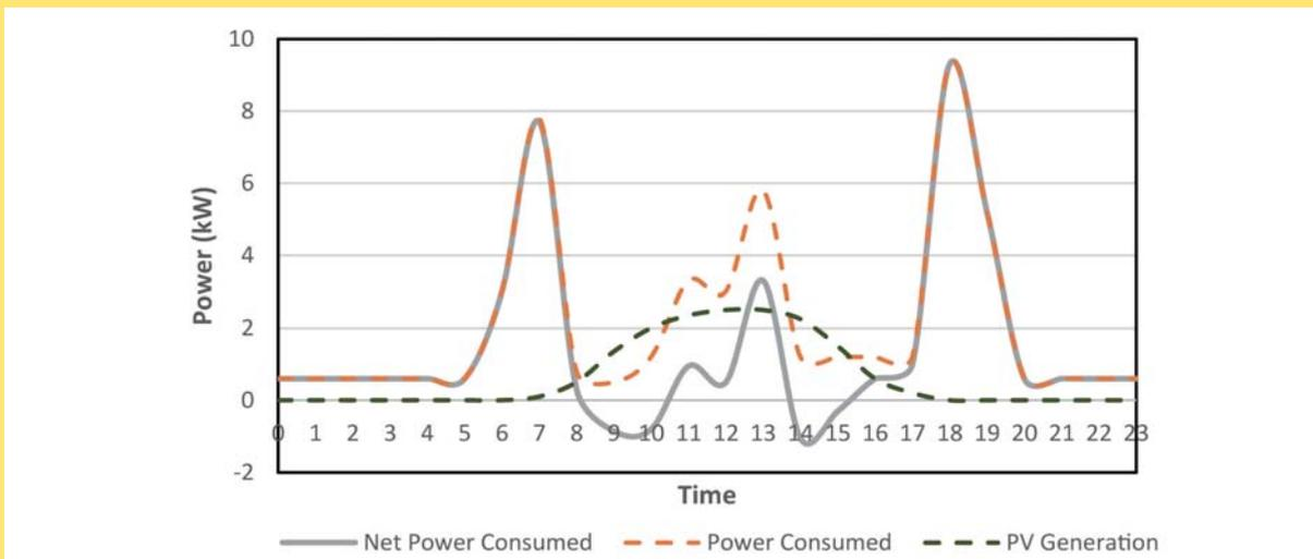
Figure 10 Electricity consumption and generation for a typical day (adapted from Doiron *et al.*, 2011)
