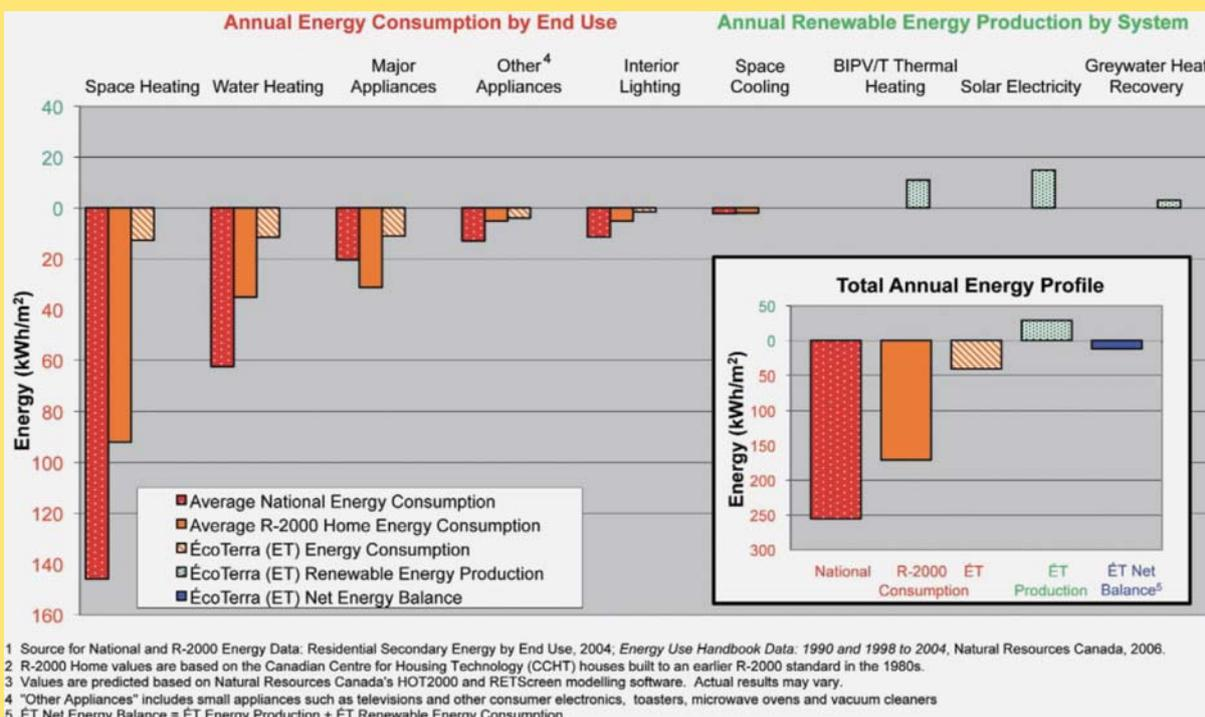
Figure 11 Annual electricity consumption and generation of the EcoTerra™ house according to energy end-uses and systems (CMHC, 2007a)
